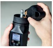
Pour the sample into the grinder and grind. The sample size is measured out in the built-in measuring cup.
