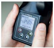
Press the test button and read the moisture content directly from the display.
